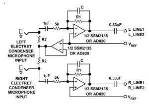
Figure 16. "Phantom-Powered" Microphone Input Circuit
